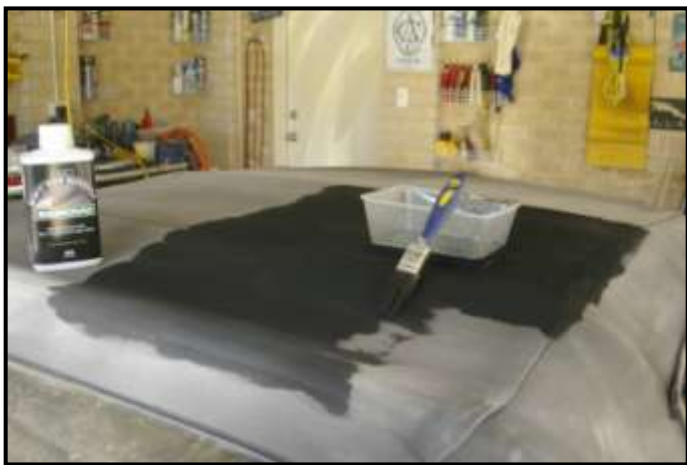
Figure 6: Application of first coat of "Reviver".
